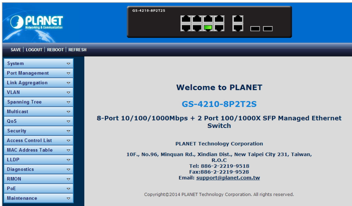
Figure 3-1-4 Web Main Screen of Managed Switch
